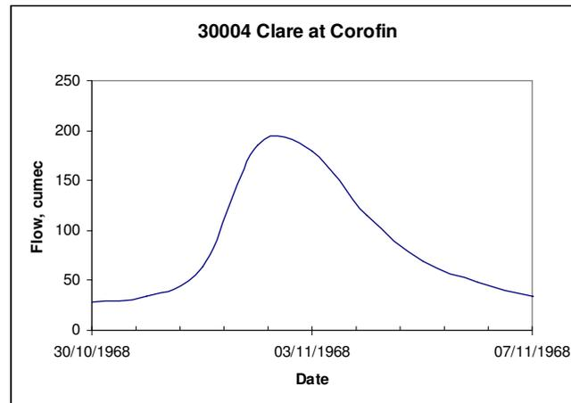
**Figure 6.** 1968 Flood Flow Hydrograph at Corofin
