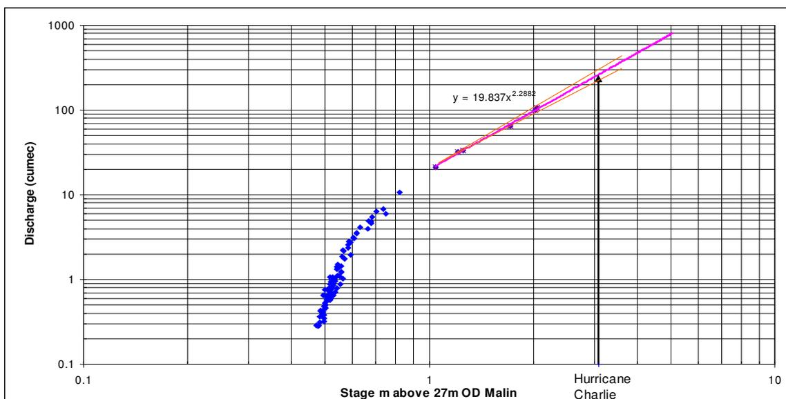
**Figure 1** Rating Data and best fit Rating Curve for River Dodder Flood Flows at Orwell Bridge (Station 09010)
