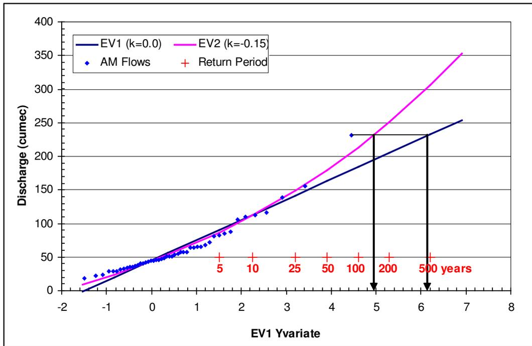
Figure 2 Dodder Flood Frequency analysis and estimate of Return Period for Hurricane Charlie Peak flow
