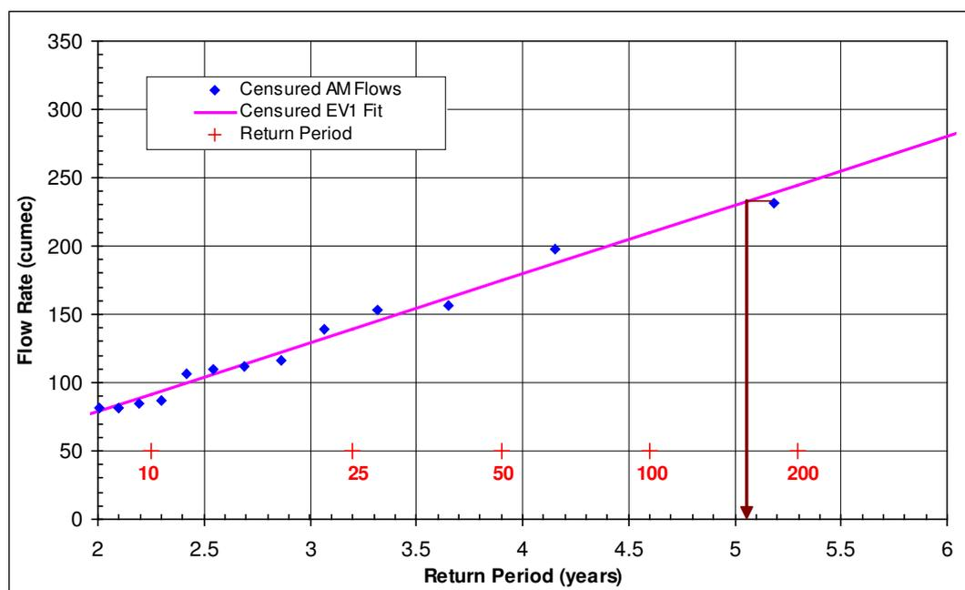
Figure 3 Censored Flood Frequency EV1 analysis using largest 15 AM flows in 100years (period 1905 – 2004).
